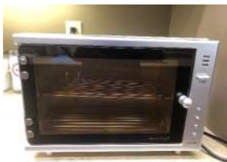
UV light sterilizer for 30 minutes. One mask can be sterilized up to 5 times.
